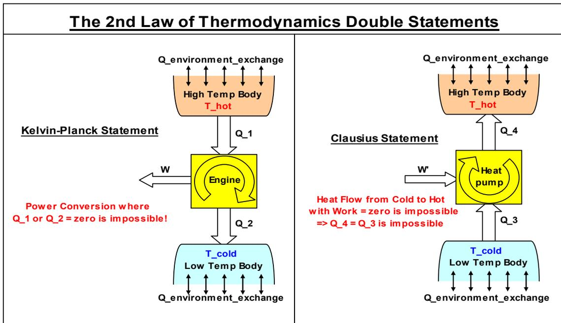
**The Clausius statement:** It is impossible to construct a device that operates in a cycle and produces no effect other than the transfer of heat from a cooler body to a warmer body. See the right-hand sketch of figure 1, above. This statement is related to the refrigerator or heat pump. In effect, it states that it is impossible to construct a refrigerator that operates without an input of work. This also implies that the COP is always less than infinity.
