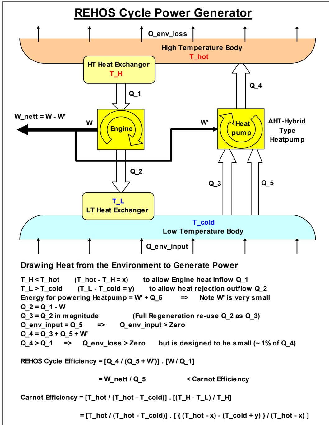
In another paper I have written, the REHOS Cycle efficiency calculated to 80,1%, while the Carnot efficiency was 90,1% with the system high temperature ( $T_{hot} = 80^\circ\text{C}$ ) and the system low temperature ( $T_{cold} = -5^\circ\text{C}$ ) extracting heat from a liquid reservoir at ambient ( $22^\circ\text{C}$ ).
