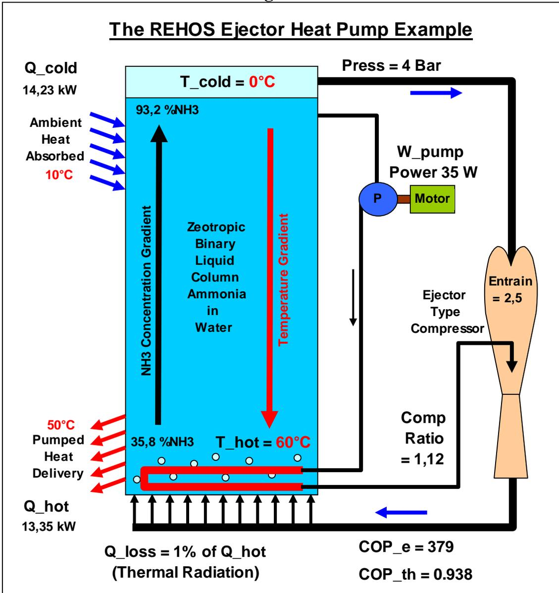
The same as before, for this Regenerative HOS heat pump, or REHOS Ejector heat pump, the definition (COP<sub>e</sub>) for cooling service is defined as:
