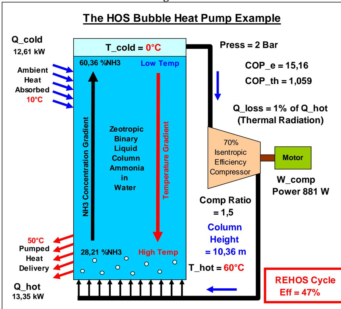
of the column where sliding temperature at a relatively constant pressure take place, very similar to the Lorenz Cycle hybrid models discussed above. The bubbling compressed vapor entering the column at the bottom also perform a vapor lift pumping action, driving the liquid counter flow circulation. During the countercurrent liquid mixture flows, both heat and species exchange would take place, enhancing the single temperature and
