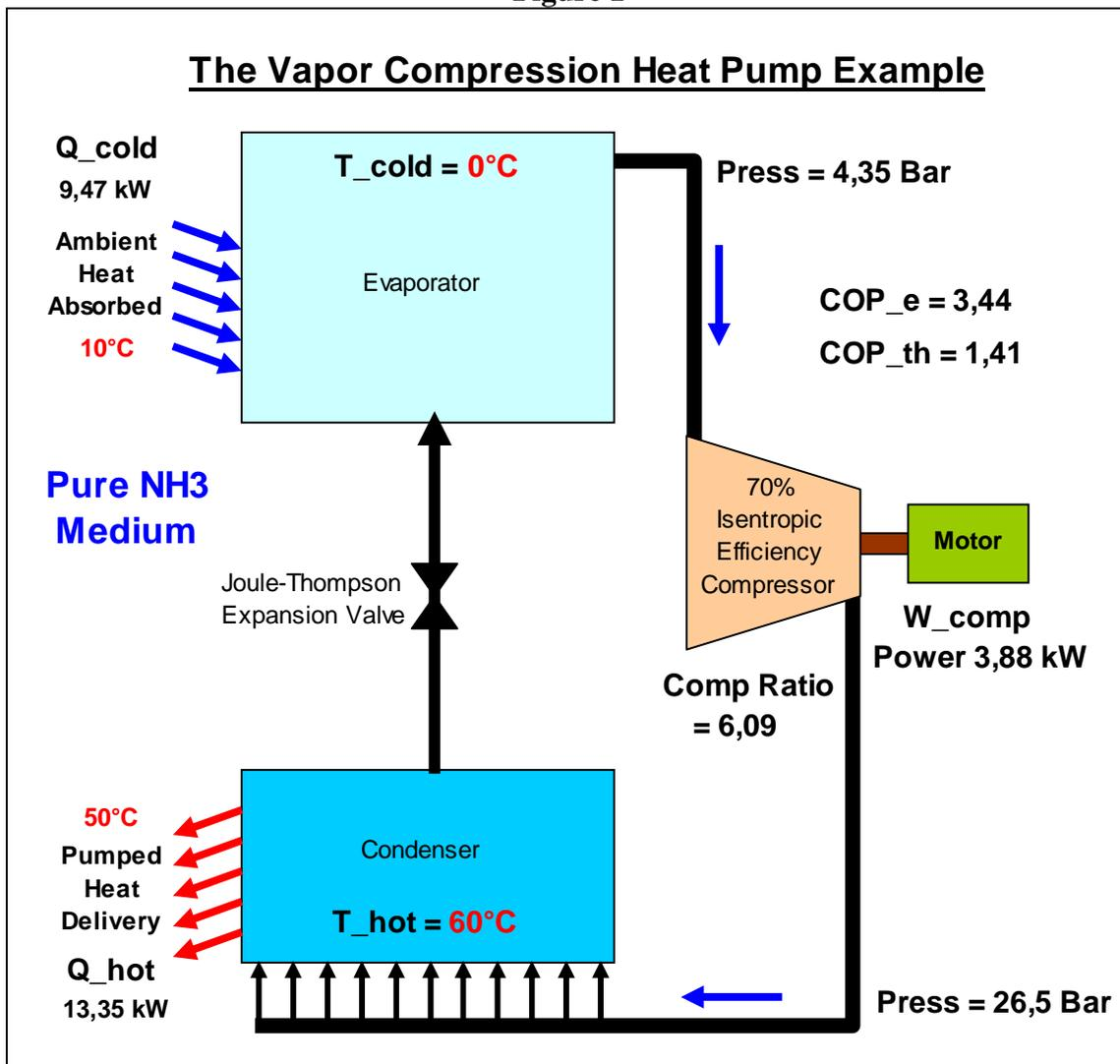
The electrical coefficient of performance (COP<sub>e</sub>) for cooling service is defined as:
