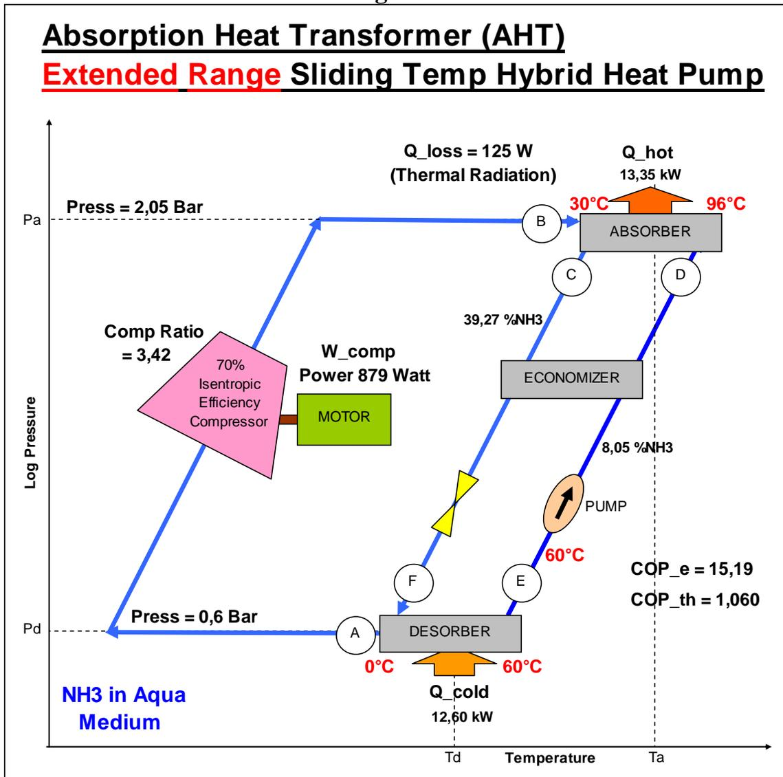
**The Extended Range Sliding Temperature AHT-VC Hybrid Heat Pump:**
