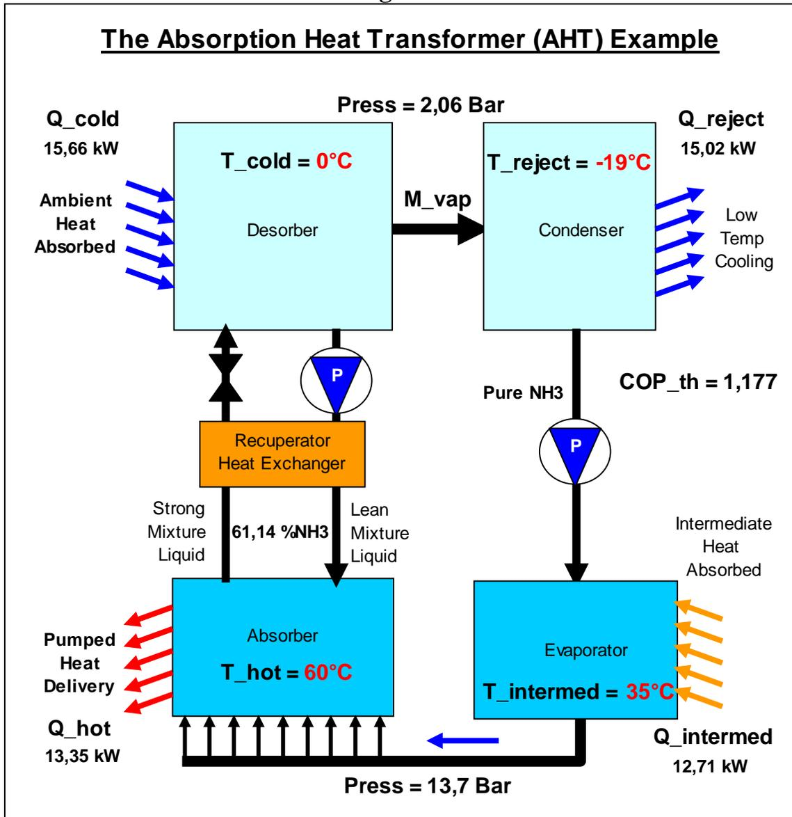
example sketched in figure 3, ammonia vapor saturated at 35°C is generated in the evaporator and is absorbed in the absorber (and heat it with the absorption heat) to 60°C, matching the 13,7 Bar pressure of the evaporator. The saturation vapor pressure of pure NH<sub>3</sub> at 60°C is 26,5 Bar, double the actual absorber pressure, demonstrating the huge pressure reduction achieved by using an absorber instead of condenser.
