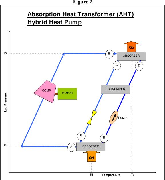
entering the desorber at line (F). The resulting weak liquid solution leave the desorber at line (E), to be pumped to higher pressure, (Pa) of the hot absorber. The pumped NH3lean solution line E -> D is also in heat exchange (economizer) contact with the NH3-rich solution line C -> F flowing from the hot absorber back to the low pressure (Pd) cold desorber.
