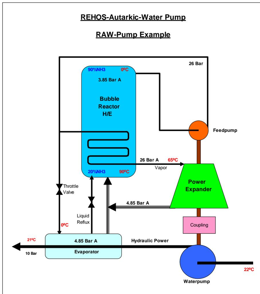
Obviously some radiant heat losses occur due to the hot components radiant heat loss, and the expander netto delivered power is also decreased as it needs to power not only the ORC liquid pump, but the heat transformer liquid pump as well. Nevertheless the REHOS cycle example designed as sketched in figure 8 operate at ~ 80% heat to power
