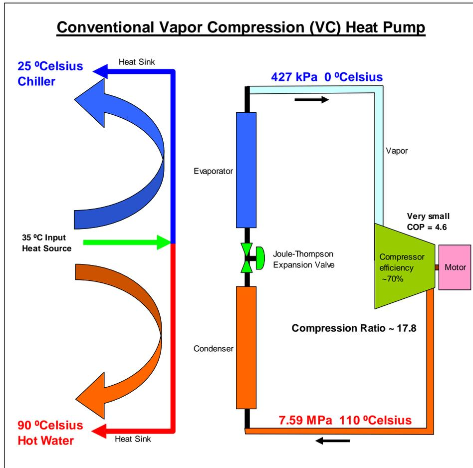
In the VC-heatpump, a suitable refrigerant vapor (eg. ammonia -NH<sub>3</sub>) is compressed to a high pressure by the compressor and is condensed at the high saturation temperature and pressure, delivering the latent heat of condensation to a heat sink at high temperature.
