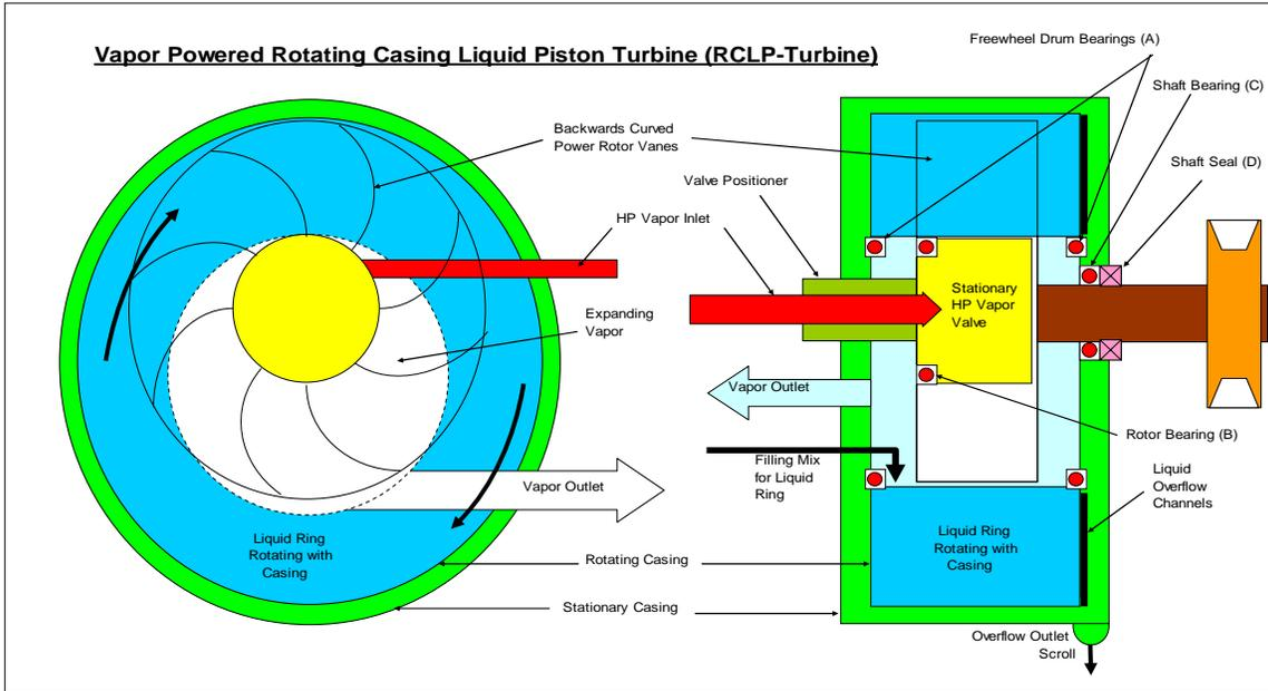
Costing of this expander would start with the cost of a simple centrifugal pump of similar power rating, doubled to account for the additional rotating casing, and further multiplied by 4 to account for other complication factors like additional bearings and balancing as well as the vapor channels and valves etc. Cost of the complete RCLP - Turbine could therefore be estimated as power equivalent pump cost x 8, namely
