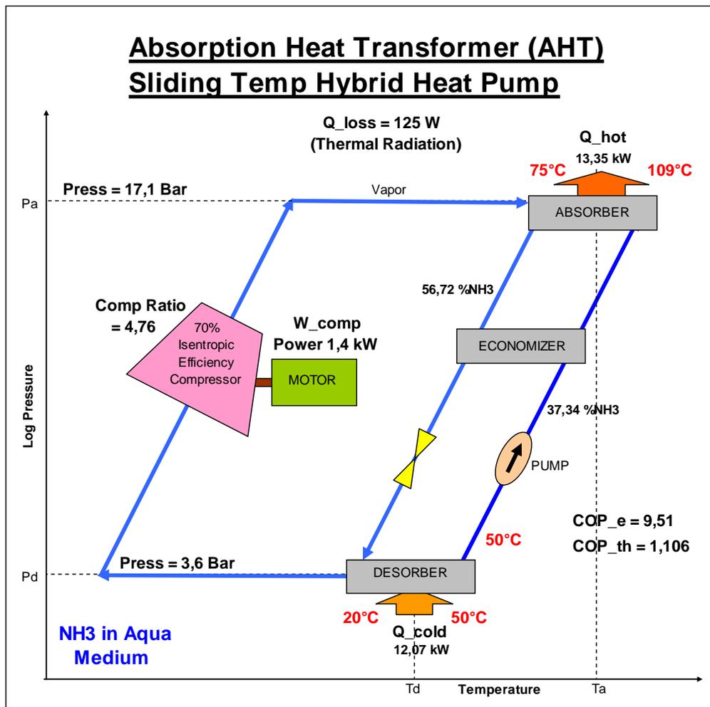
Nordtvedt also paved the way for the comprehensive development and testing of the compression/absorption heat transformer (CAHT) reported in 2014 by Anders Borgås in his thesis [7]. He developed the CAHT using temperature glides of 50°C in the absorber and 40°C in the desorber. His experiments and simulations of heating water from 110°C
